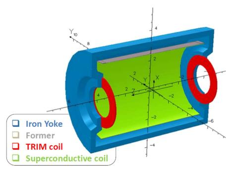
The MPD Magnet is a single solenoid more than 7 m long and with a diameter of about 5 m. The cable (custom designed on purpose) is manufactured by coextrusion of stabilizing high-purity aluminum and superconducting NbTi strand. The coil solenoid has an indirect cooling system that consists in a hydraulic LHe circuit welded directly on the coil former.
